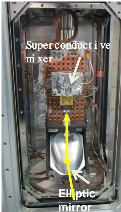
Inside of the Cryostat
