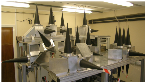
Conical beam dumps in the 94GHz pulsed ESR spectrometer "HIPER" (Rev. Sci. Instr. 80, 103102, 2009)
