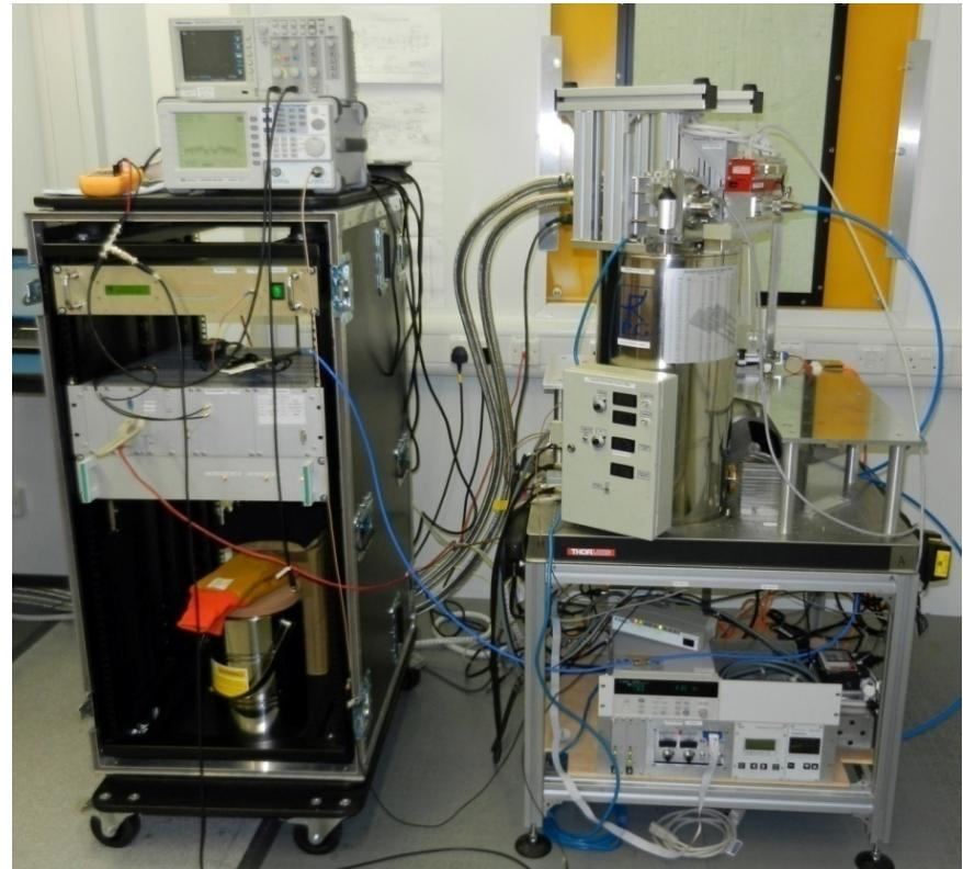
*A microwave radiometer for the remote sensing of nitric oxide and ozone in the middle atmosphere, Espy et al, Proc. SPIE 6362, 63620P-3 (2006).*
