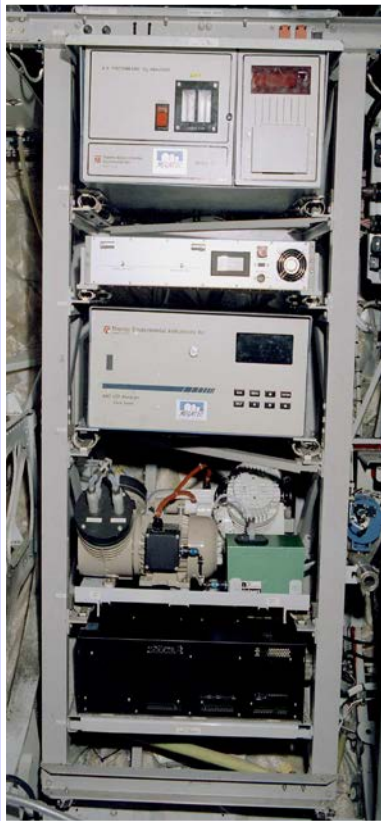
Instrumentation in Avionic Bay below the cockpit O_3/CO/H_2O/NO_y/DAS
