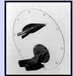
Inlet tubes On the Aircraft Fuselage
