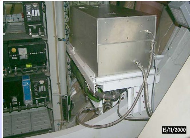
Instrumentation in Avionic Bay below the cockpit O_3/CO/H_2O/NO_y/DAS
