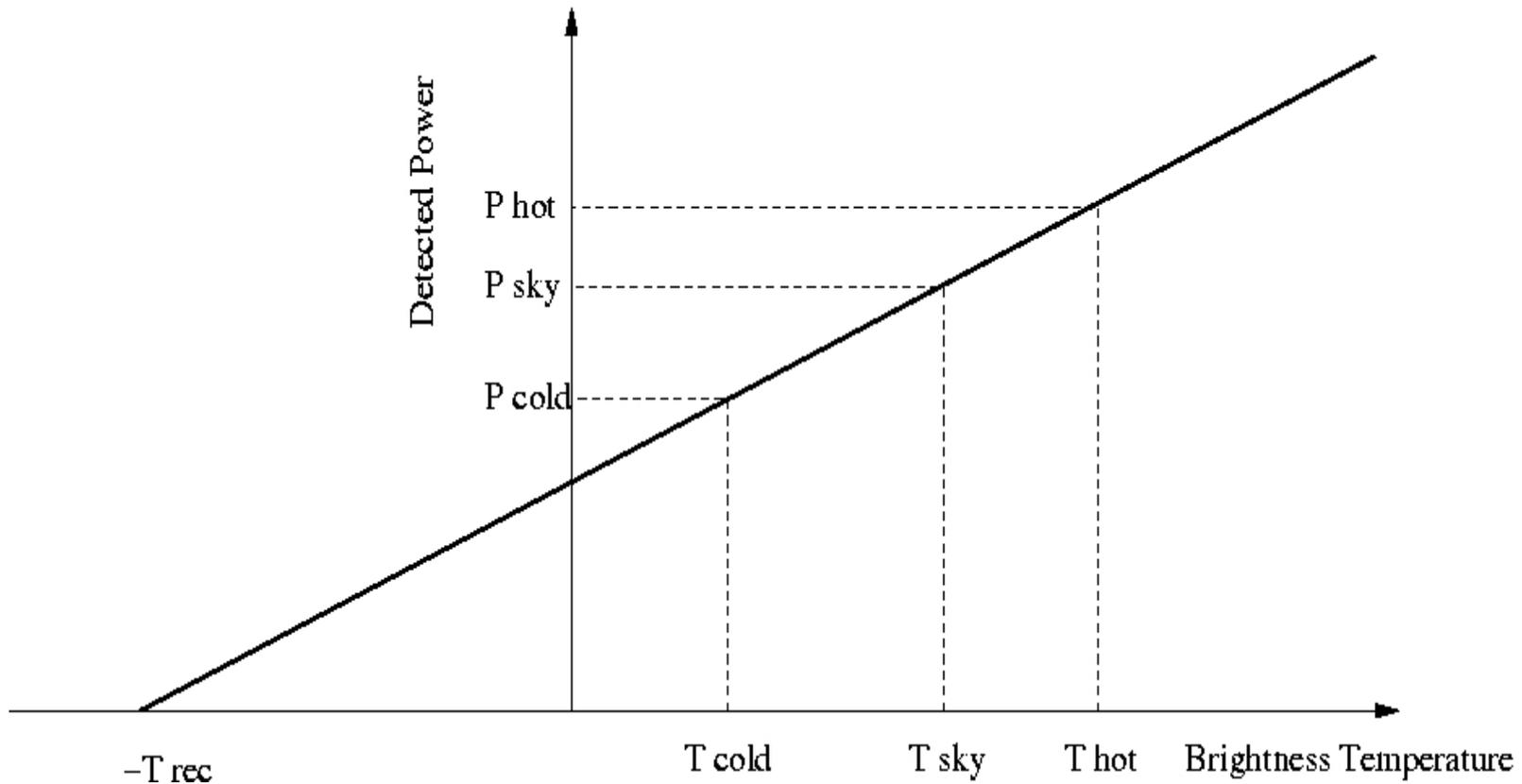
$$T_{sky} = \frac{P_{sky} - P_{cold}}{P_{hot} - P_{cold}} (T_{hot} - T_{cold}) + T_{cold}$$
